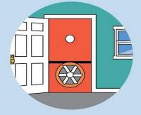
Contact a professional to check for air leaks with a blower door test.
